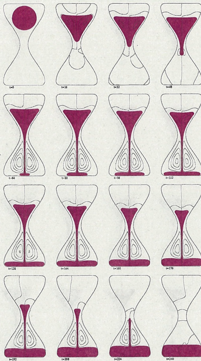
Figure 3: Interfaces and streamlines at t = 0, 16, \dots, 240 subject to the non-slip boundary conditions.
